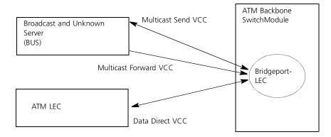
Figure 2-8 Data VCCs in ATM Backbone SwitchModule LAN Emulation
